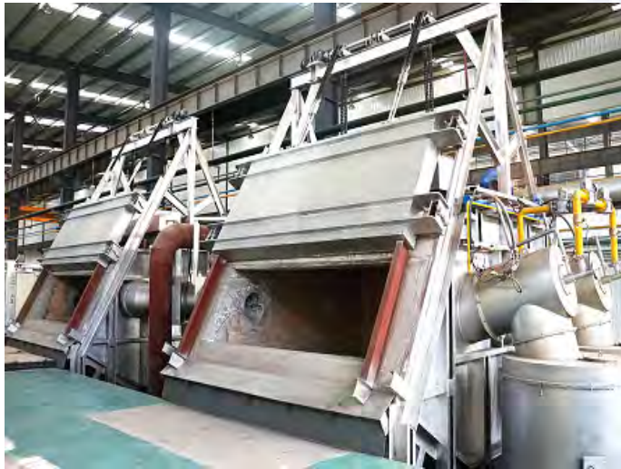
15T rectangular gas-fired aluminum melting furnace
