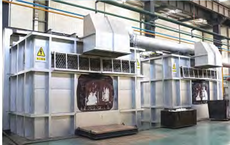
5 tons of electric heating rectangular aluminum melting furnace
