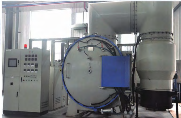
Vacuum Brazing Furnace
